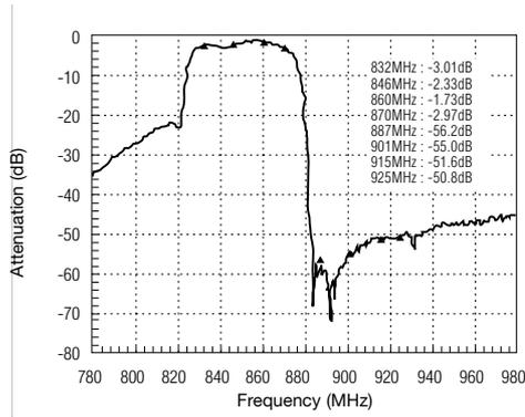
Fig. 8 Attenuation characteristics of receiving filter based on a circuit composition with attenuation poles
