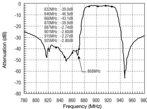
Fig. 3 Attenuation characteristics of a transmitting filter based on a conventional circuit composition with attenuation poles
