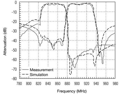
Fig. 13 Attenuation characteristics and simulation results of SAW antenna duplexer for Japan CDMA system.
