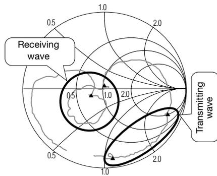
Fig. 12 Impedance characteristics of transmitting filter only
