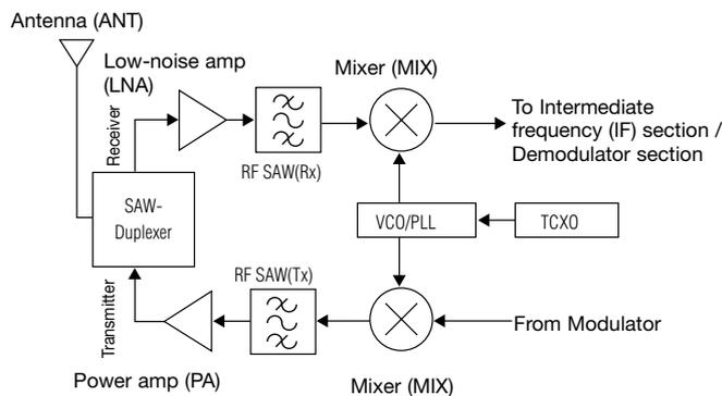
Fig. 1 Block diagram of radio frequency section in mobile phones
