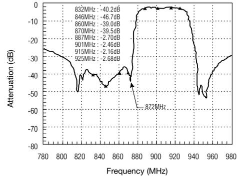
Fig. 5 Attenuation characteristics of a transmitting filter based on a new circuit composition with attenuation poles
