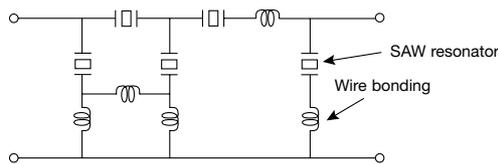
Fig. 4 New circuit composition with attenuation poles providing sharp attenuation characteristics on low frequency side of pass band
