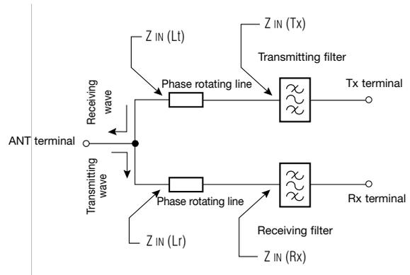
Fig. 9 Composition of SAW antenna duplexer
