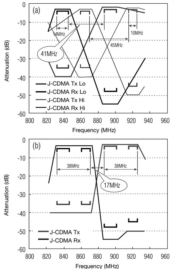
Fig. 2 Comparison of attenuation band in Japan CDMA band dividing type (a), and full-band type (b)
