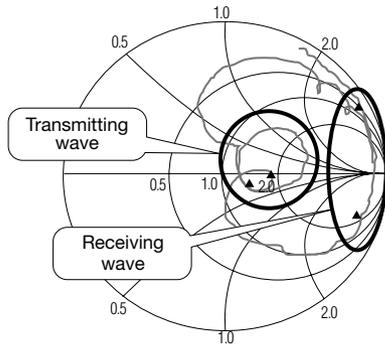
Fig. 11 Impedance characteristics of phase rotating line and transmitting filter only
