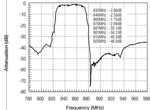
Fig. 6 Attenuation characteristics of a receiving filter based on a SAW resonator
