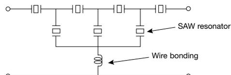
Fig. 7 Circuit composition with attenuation poles achieving high attenuation on high frequency side of pass band
