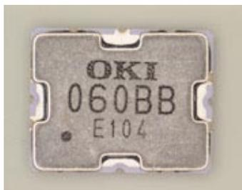
Photograph 1 SAW antenna duplexer for Japan CDMA system
