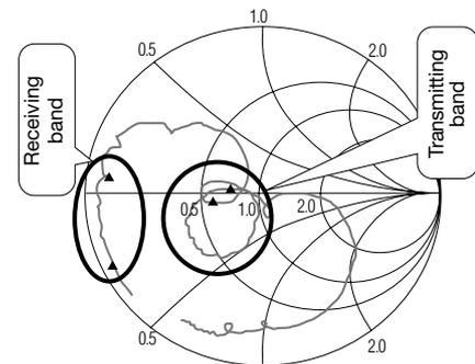
Fig. 10 Impedance characteristics of transmitting filter only
