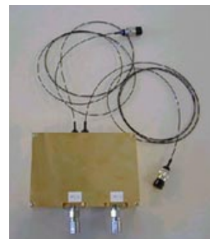
The OTDM MUX module is a basic building block for a return-to-zero (RZ) or a soliton transmitter and operates at 40 gigabits per second (or OC-768 standard). The module multiplexes two 19.9-gigabit-per-second electrical non-RZ signals and converts to a 39.8-gigabit-per-second optical RZ signal.
