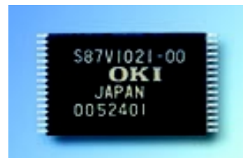
The MS87V1021 voice recorder incorporates a 2-megabit DRAM, Micro Controller Unit (MCU) and analog circuit.
