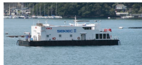
Our stationary measurement barge, Japan's only underwater acoustics measurement facility
