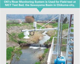
For one test bed site prepared by the National Institute of Information and Communication Technology (NICT), we developed and delivered a river monitoring system that enables remote monitoring of river water levels using a wireless 920 MHz band multi-hop network to collect data via sensors for tracking water levels and rainfall amounts.
