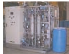
● Conservation of Water Resources Using a Recycling System for Surface Active Agents (Example from Fiscal 1998)
