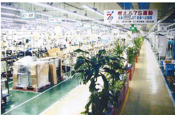
Efficient use of production plant space and a reduction in the ceiling lights (Oki Electric Honjo District)
