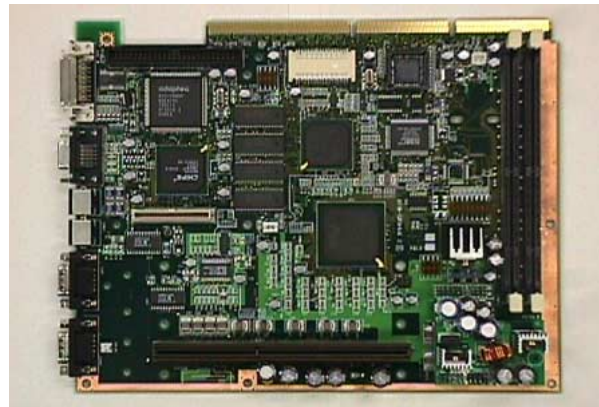
A printed circuit board with electronic components connected by lead-free solder
