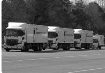
Automatic driving and queue driving with 4 meter gaps between vehicles
