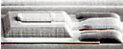
A thin-film LED bonded to a driver IC using EFB technology
