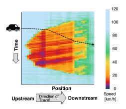
Figure 2. Visualization of Traffic Probe Data
