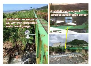
Figure 3. Installation on Railway Bridge
