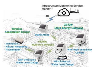
Figure 1. System Configuration
