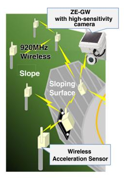
Figure 5. Configuration Example of Slope Monitoring System
