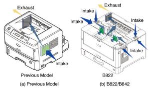
Figure 5. Internal Cooling Configuration
