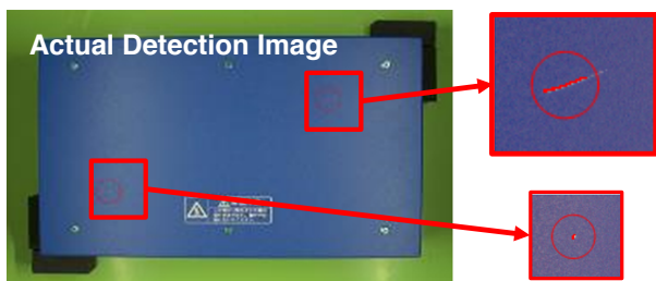
Figure 3. Scratch Detection of Top Cover
