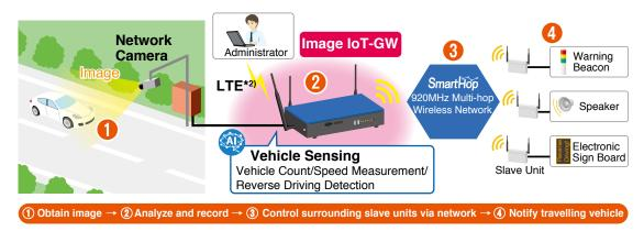
Figure 2. Warning through AISION Vehicle Sensing System and External IoT Device Interworking
