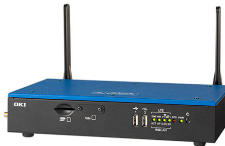
Photo 1. Example of Edge Processor (OKI's AI Edge Computer AE2100 6) )
