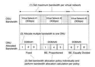
Figure 7. Example Configuration for Domain DBA
