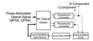
Figure 2. Basic Configuration of Optical Phase-Locked Circuit
