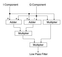
Figure 5. Calculation Required for Phase Error Extraction in QPSK
