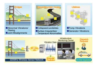
Figure 1. Social Infrastructure Monitoring System Utilizing 920MHz Wireless Sensor Network
