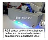
Figure 9. Automatic Print Adjustment Mechanism
