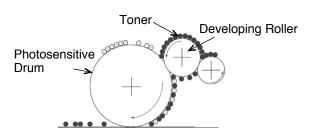
Figure 9. Single-Component Contact Development System
