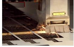
Photo 4. Contour Cutting using a Laser
