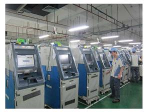
Photo 8. Final Inspection of ATM-Recycler G7
