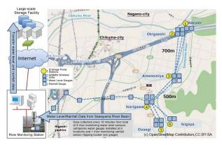
Figure 3. Configuration of System Installed at Sawayama River, Chikuma-city
