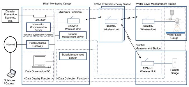
Figure 1. Configuration of River Monitoring System
