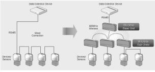
Figure 4. RS485 Transmission Model
