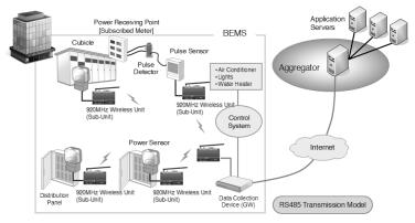
Figure 8: Configuration Example: BEMS
