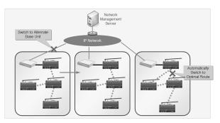
Figure 2. Dynamic Routing Function
