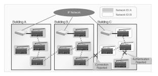
Figure 1. Independent Network Configuration
