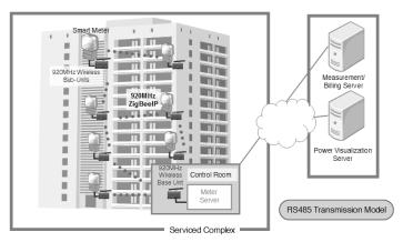
Figure 9. Configuration Example: MEMS
