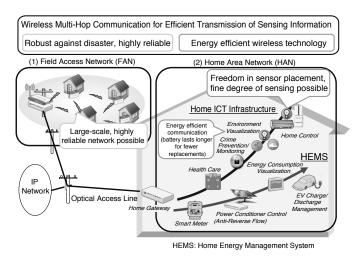
Figure 3. Features of a Smart Network
