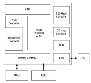
Figure 4. Block Diagram of Green ASIC
