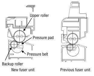
Figure 3. Fuser Unit Cross Sections
