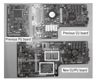
Figure 5. Comparison of Control Boards
