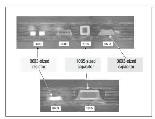
Figure 2. Mixing Chip Components with Different Sizes
