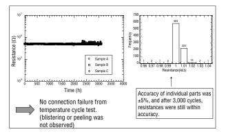
Figure 6. Result of Temperature Cycle Test
