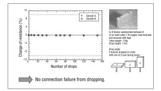
Figure 5. Result of Drop Test
