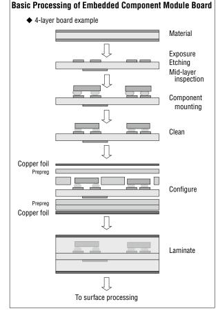
Figure 3. Embedded Component Module Board Manufacturing
