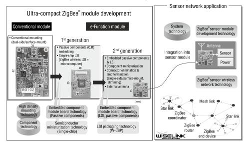
All required elements for the function module provided with one stop.
