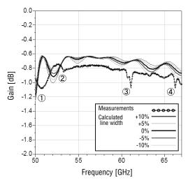
Figure 9. Dependence on Transmission Line Width and Measurement Results
