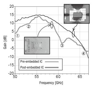
Figure 10. Small-signal Gain Characteristics
