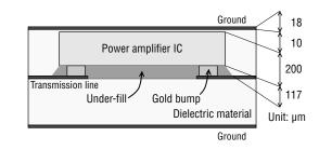
Figure 4. Cross-section of Embedded IC Printed Circuit Board
