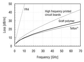
Figure 1. Loss Comparison of Printed Circuit Boards
