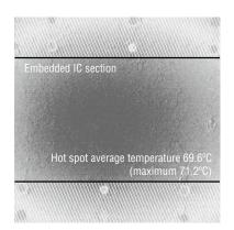
Figure 11. Temperature Distribution of Board Surface
