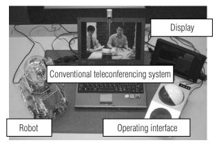
Fig. 2 System configuration diagram
