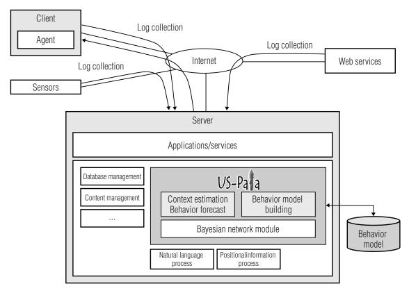
Fig. 2 Overall configuration of US-PALA engine
