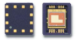
Photo 1 QFN package (pin pitch: 1.0 mm)
