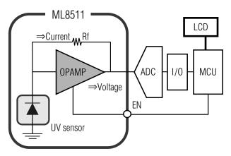
Fig. 2 Example of configuration for UV meter using ML8511
