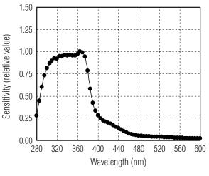
Fig. 1 Spectral sensitivity characteristics
