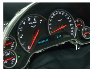
Photo 1 Example of application for automotive instrument panel (provided by Nippon Seiki Co., Ltd.).
