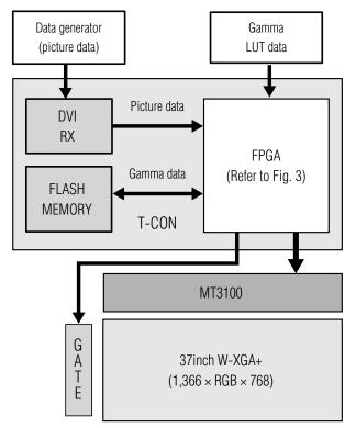
Fig. 4 Block diagram of demonstration system
