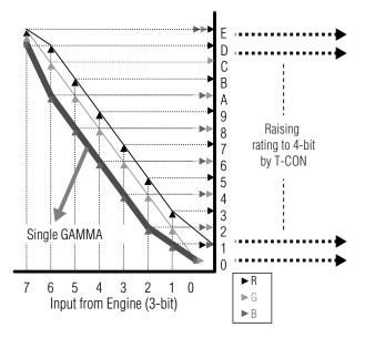
Fig. 2 Generation of data for independent RGB gamma
