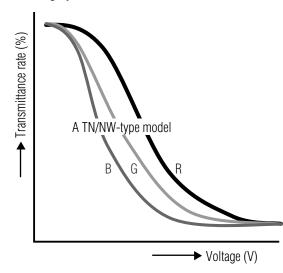
Fig. 1 VT characteristics that vary individually for RGB (gamma)
