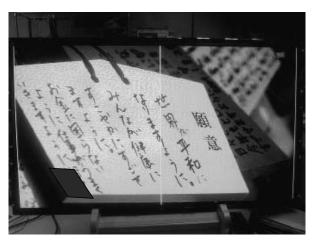
Photo 2 Actual image on panel (right half is image with individualized gamma compensation for RGB)
