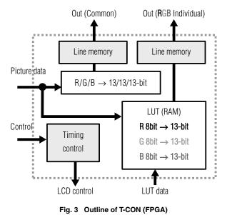
Control signals, such as the start pulse sent to the gate driver and source driver used for controlling screen scans, are generated in the Timing Control section.
