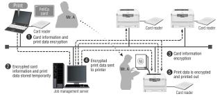
Fig. 3 Secure printing feature
