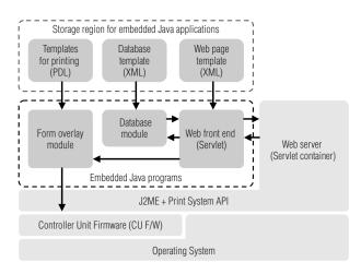
Fig. 5 Serverless on-demand printing configuration
