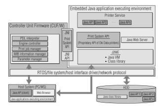
Fig. 1 System configuration of embedded Java applications
