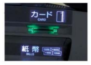
Fig. 2 Example of optical guidance
