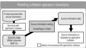
Fig. 3 Example of software operation using ProtecPaper SDK
