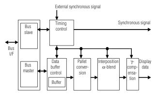
Fig. 2 Block diagram of display controller
