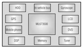
Fig. 1 An example of an application for audio visual navigation and communication integrated system.
