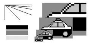
Fig. 4 Graphic function example Left top : Imaging straight lines. Left bottom : Fills. Right : Magnification and reduction.
