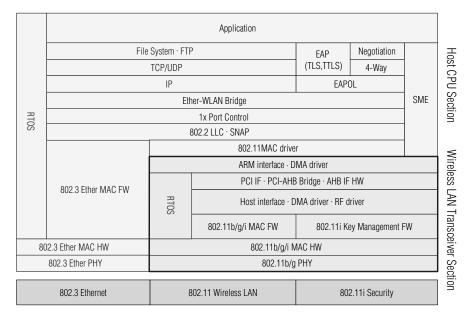
FIg. 4 Protocol Implementation Example for Wireless LAN and Wired LAN.
