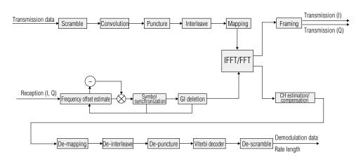
FIg. 2 Block diagram of the 802.11a/g PHY BB signal processing IP.
