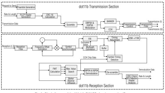
Flg. 3 Block diagram of the 802.11b PHY BB signal processing IP.
