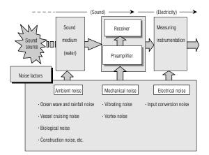
Fig. 1 Noise factors relating to hydroacoustic measurements.
