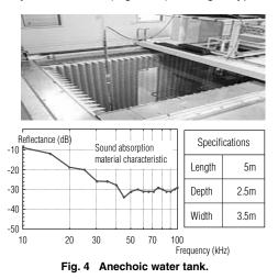
absorbing resin materials are attached to the internal surface of the water tank, which makes it possible to conduct measurements in conditions where no reflections from the internal surface of the water tank exist for frequencies of approximately 30KHz and above.
