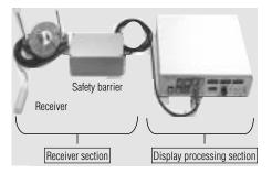
Fig. 8 Configuration of a Sonic Tester.
