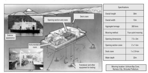
Fig. 2 Marine instrumentation barge (Seatec II).
