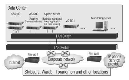
Fig. 2 Company-wide IP-Centrex system
