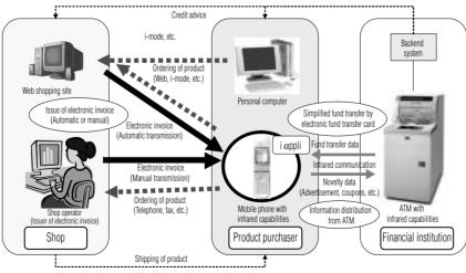
Fig. 3 Prototyped mobile electronic invoice system
