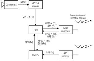
Fig. 4 System block diagram of the IVPC system for moving image transmissions
