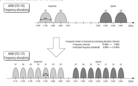
Fig. 1 Frequency allocation for the DSRC-type RVC system
