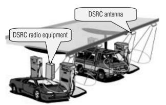
Fig. 7 System for self-service filling stations
