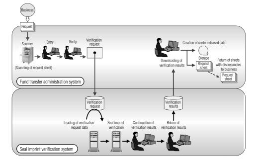
Fig. 3 Overview of fund transfer system and seal imprint verification system linkage
