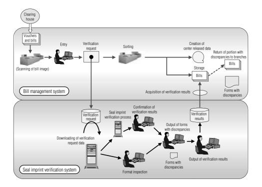
Fig. 4 Overview of bill management system and seal imprint verification system linkage
