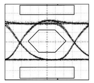
Fig. 3 155 Mb/s OLT optical output waveform
