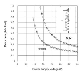
Fig. 3 Comparison of performance in 4NAND vertically integrated transistor
