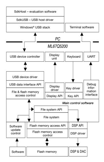
Fig. 2 Software structure
