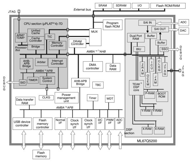
Fig. 1 System structure
