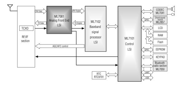
Fig. 3 Block diagram of third-generation mobile communications terminal equipped with Oki system LSIs
