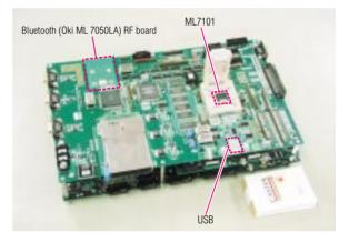
Photo. 1 Control platform evaluation board
