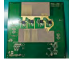
Millimeter wave antenna and RF boards
