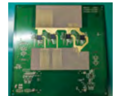
Millimeter wave antenna and RF boards
